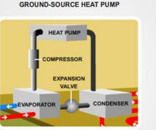
The ground loop absorbs heat from the ground. The heat is transferred to a refrigerant by the evaporator, changing it from a liquid to a gas. The compressor compresses the gas, causing the temperature to rise. The condenser then transfers the heat from the hot gas to the central heating system.
